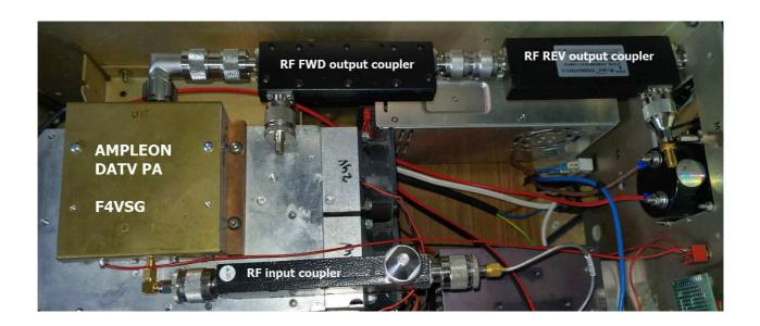
I am using one input coupler and 2 output couplers. FWD & REV.
